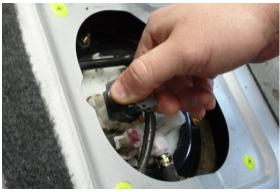
3. Using light oil, lubricate the O-rings on the adapter fittings (not included).
