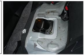
2. To depressurize the fuel system, first squeeze the tab and unplug the gray wiring connector on top of the pump housing (shown). Start the engine and allow it to stall. Remove the key from the ignition. Unscrew the gas tank filler cap temporarily to relieve any residual pressure.
