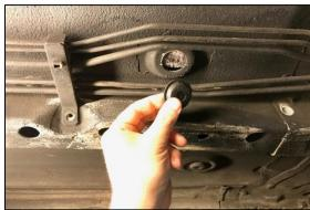
8. Flip the plug around and reinsert until it locks in place, as shown. This will provide additional room for the fuel filter assembly.
