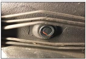
9. Lineup the filter bracket assembly to the open threaded holes. Install the 3 provided button head bolts to the chassis. If necessary, pull and spread the OEM hard lines to permit additional space.
