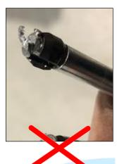
If any damage is found remove pad pin and replace.
