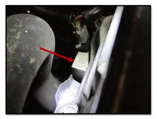
3. Using a Racket with 6mm Allen Bolt Head and the M8 x 20mm Bolt supplied, bolt the heat shield to the car.
