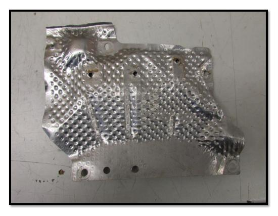
5. Bolt this section of the original heat shield back into the car using only the bottom two bolts (Circled). **Note:** Leave the top bolt out at this stage.
