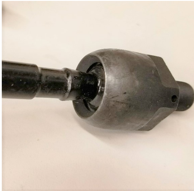
Figure 3: Dry tie rod before grease being packed into it.
